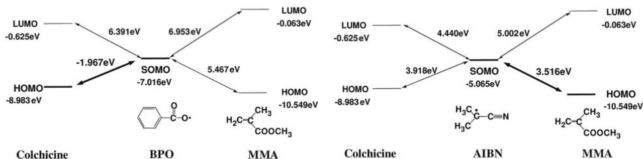
Figure 2. The energy levels of the SOMO of BPO and of the HOMO and LUMO of colchicine.
