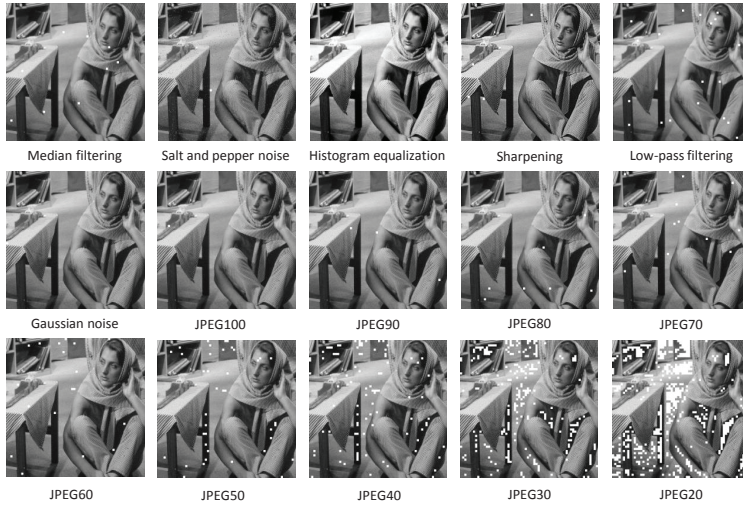
Figure 12. Results obtained with semifragile watermarking. The white squares indicate non-detected blocks.
